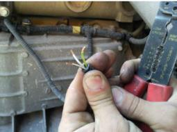
**5-** Install the gaskets and terminals to the wiring.
