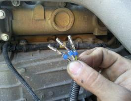
**6-** Fit the wiring to the connector and install the gasket on the free slot.
