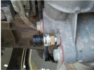
4- Remove the old connector from the wiring and remove the cover of the wiring,
